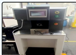
30T Servo Terminal Crimping Machine - upto 120 sq mm
