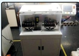
Auto Cable cut strip mc - upto 120 sq mm
