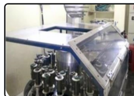
Braiding M/c (36- Spindle, 3-16mm)
